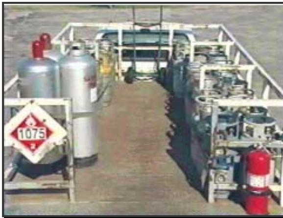
Figure 5.1.6b – Vertically Secured Cylinders
