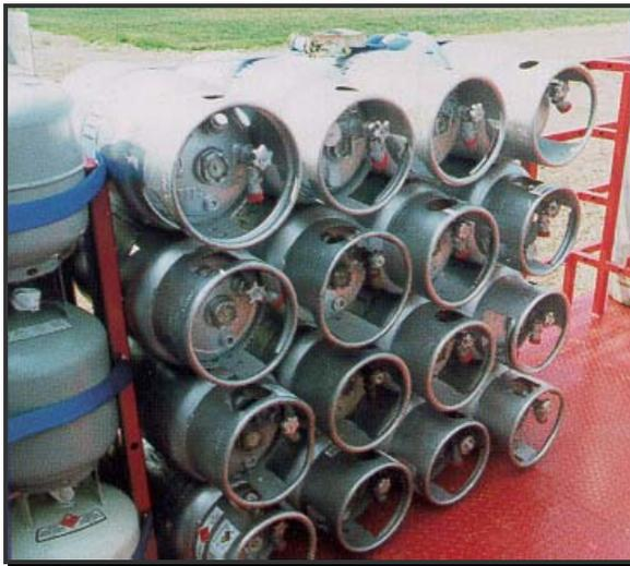
Figure 5.1.6c – Horizontally Secured Cylinders (Relief Valve at Top)
